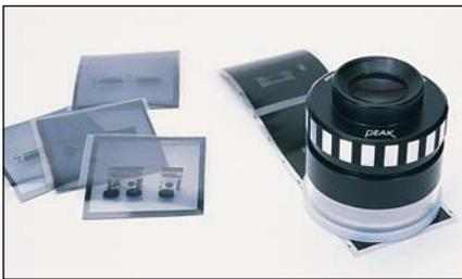
Anastigmatic loupes are known for extremely sharp center-to-edge clarity and the entire field may be viewed by merely moving the eye. High-resolution achromatic lens system with focusing from -2 to +2 diopters. Comes with measuring reticle that covers a 2" range in .005" increments. Fully coated for color corrected, flat field viewing. Smooth helicoid twist-focus mechanism is similar to the focus on
