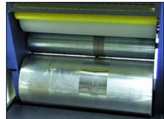
Back off the pressure at least 0.1 mm more than paper thickness and run a few sheets through the press. Increase pressure by small increments until a perfect perforation is achieved.
