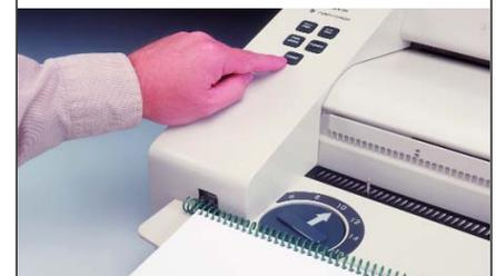
Finish the process with a powered crimp/cut on both ends of the UniCoil-bound document.
