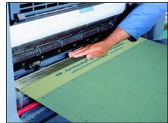
Simply mount the PPP-foil as a regular blanket. Put the PPP-base set underneath the foil and tighten to the recommended specifications.
