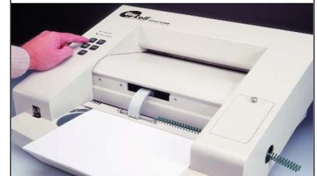
Lower guide comb and insert UniCoil® into feed for simple automatic insertion.
